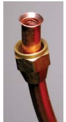
⌘ A completed flare produced with a drill bit flaring and heat. Image courtesy of Copper Development Association.
