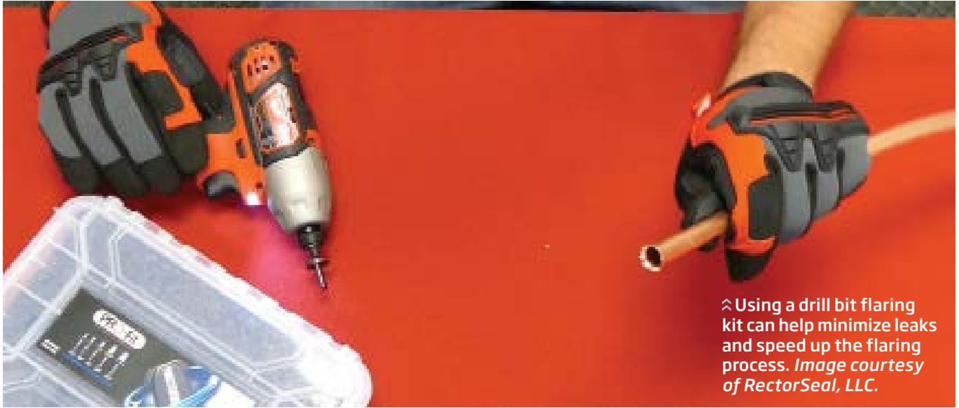
⌘ Using a drill bit flaring kit can help minimize leaks and speed up the flaring process. Image courtesy of RectorSeal, LLC.
