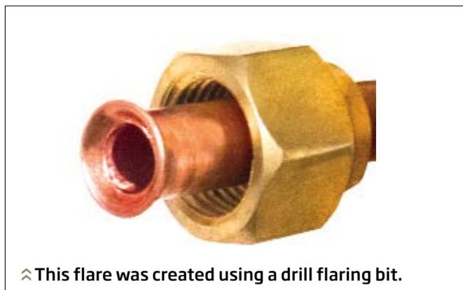
⤴ **This flare was created using a drill flaring bit.**
