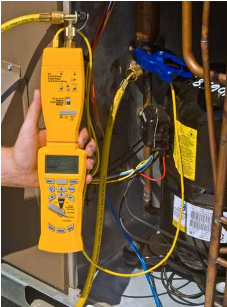
« Digital gauges are often called digital system analyzers because they allow technicians to calculate superheat and subcooling—and sometimes numerous other functions—via their ability to accurately read actual refrigerant temperature and the refrigerant's saturation temperature.
