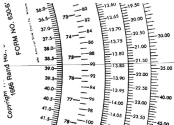
FIGURE 6. Cursor over dry-bulb temperature lines up with correct wet-bulb temperature
