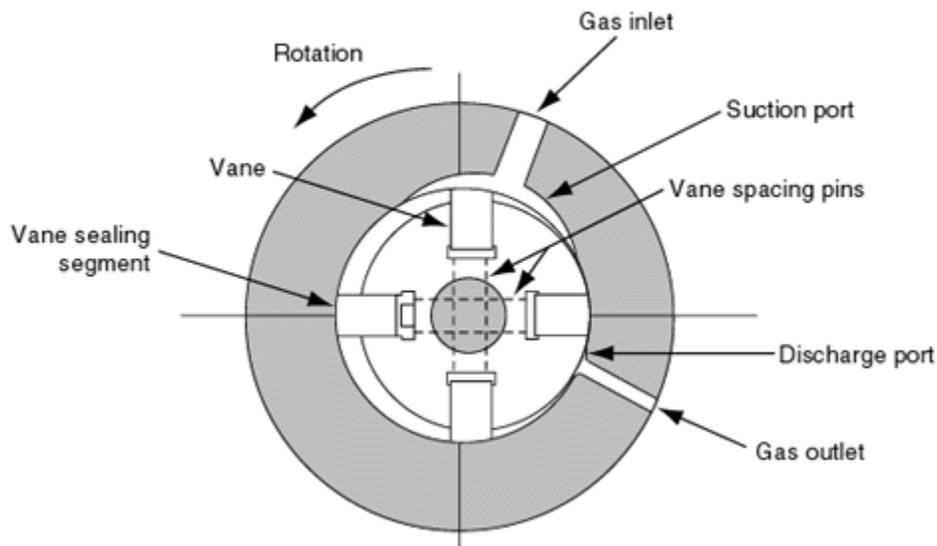
*Cross-Section of a Vane Type Rotary Compressor*
