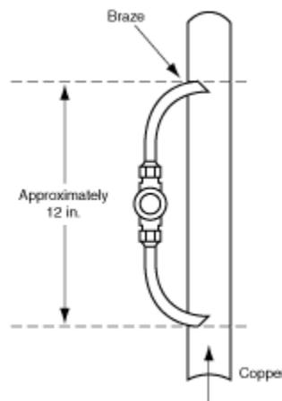
Figure 66F19B Sight glass connections for large copper tube and steel pipe lines.
