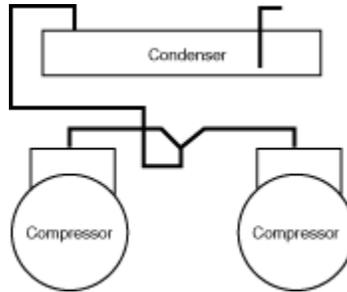
Figure 66F03C Similar connections to those in Figure 66F03B, except one hot gas line is used for both compressors. Note use of Y connections and trap.
