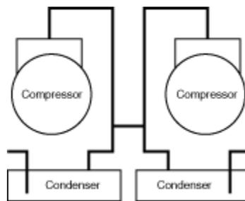
Figure 66F01 Paralleling Condensing Units
