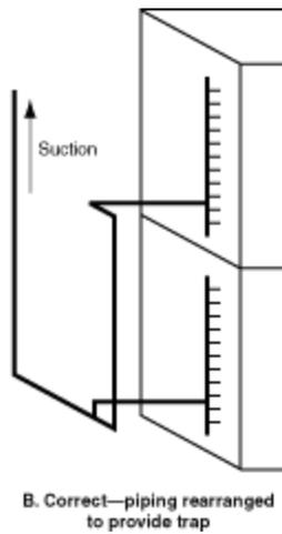
Figure 66F09B Suction piping of Figure 66F09A rearranged to provide trap (Right).
