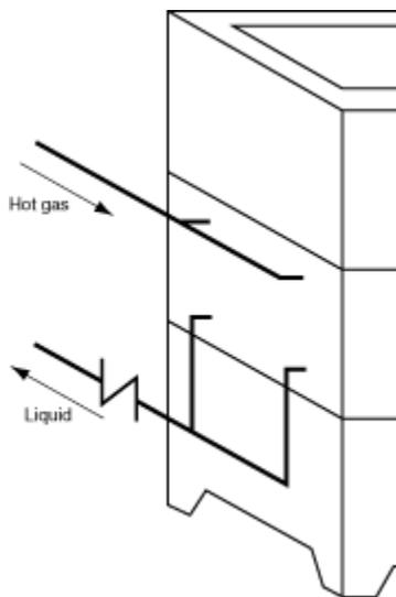
Figure 66F04B Correct hot gas and liquid lines for two section evaporative condenser.
