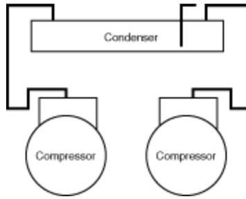
Figure 66F03C Separate hot gas lines from compressors to one condenser at a higher level, showing traps to prevent oil, and refrigerant from running back down into the compressor heads when the compressors stop.
