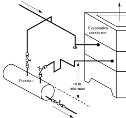
Figure 66F05 Evaporative condenser should be at higher level than its receiver. Note trap in liquid line and equalizer from top of receiver to hot gas line.
