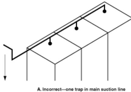
Figure 66F08A Suction line from three adjacent refrigerators with trap in main line (Wrong).
