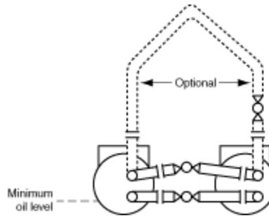
Figure 66F19A Oil and Gas equalizing lines between compressors in parallel.
