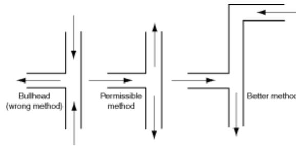
Figure 66F02C Bullhead (Wrong) and two permissible connections for paralleling two hot gas lines.
