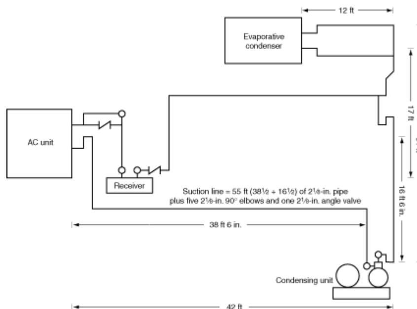
Figure 66F16 Typical 15 HP air-conditioning installation with dimensioned piping layout.
