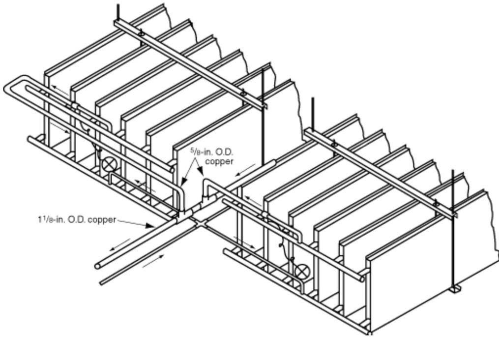
Figure 66F10C Piping layout for two parallel banks of vertical overhead plate coils.
