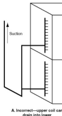
Figure 66F09A Upper coil of two evaporators in parallel can drain into lower coil (Wrong).
