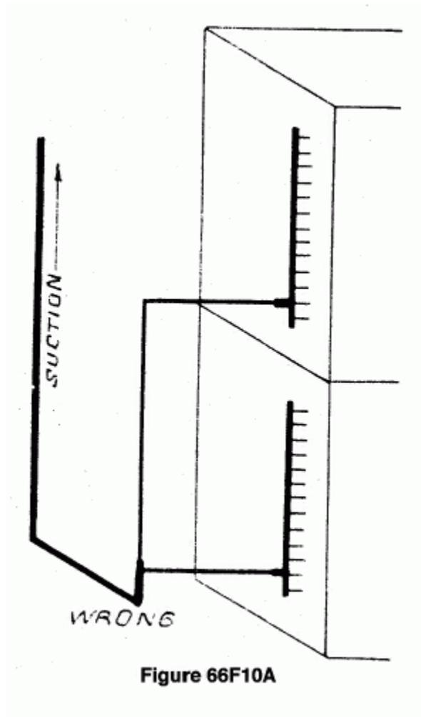
Two air-conditioning coils stacked in a vertical bank. Upper coil can drain into lower (Wrong).
