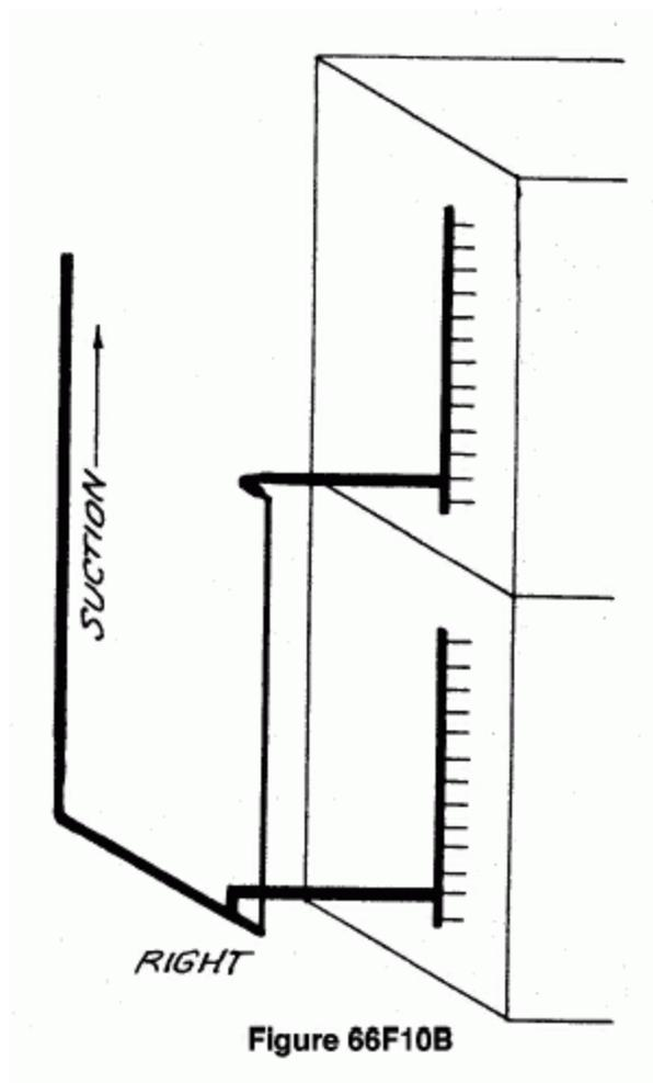
*Piping of Figure 66F10A rearranged to provide trap (Right).*
