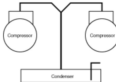
Figure 66F02A Y connection for paralleling the hot gas lines from two compressors to a condenser at a lower level (right).
