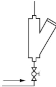
Figure 66F06B Stop valve directly below strainer in vertical liquid line (Wrong).
