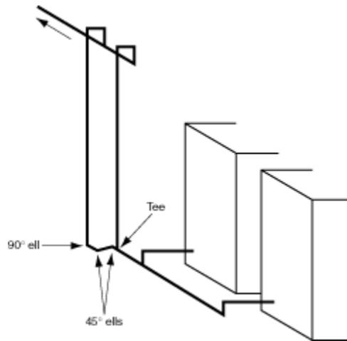
*Figure 66F11 Two vertical parallel sections of a suction line from two evaporators in multiple operated by condensing unit at higher level and provided with capacity reduction as load decreases.*
