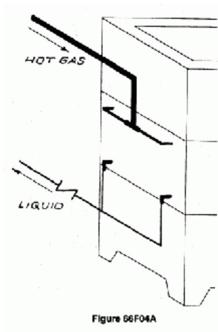
Figure 66F04A Bullhead tee connection (wrong) of hot gas line to two sections of evaporative condenser. T connection (right) of liquid lines. Note check valve in main liquid line to receiver.
