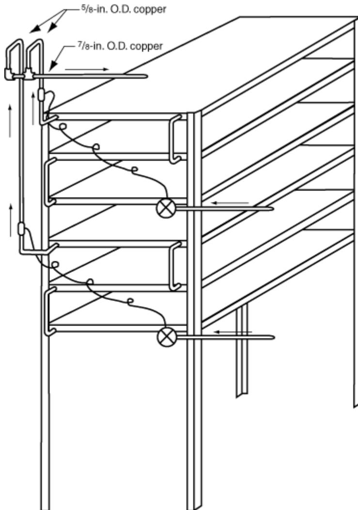
Figure 66F10D Piping layout for two parallel banks of horizontal plate coils in rack.
