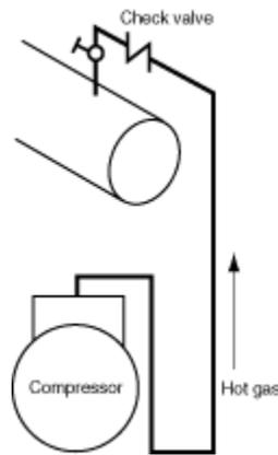
Figure 66F03D Use of check valve in hot gas line with condenser above the compressor if compressor is in cooler location than condenser.
