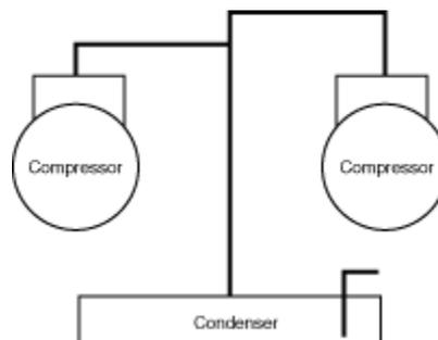
Figure 66F02B T or offset connection for paralleling the hot gas lines from two compressors to a condenser at a lower level (right).
