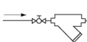
Figure 66F06D Stop valve ahead of Y strainer in horizontal liquid line (Right).
