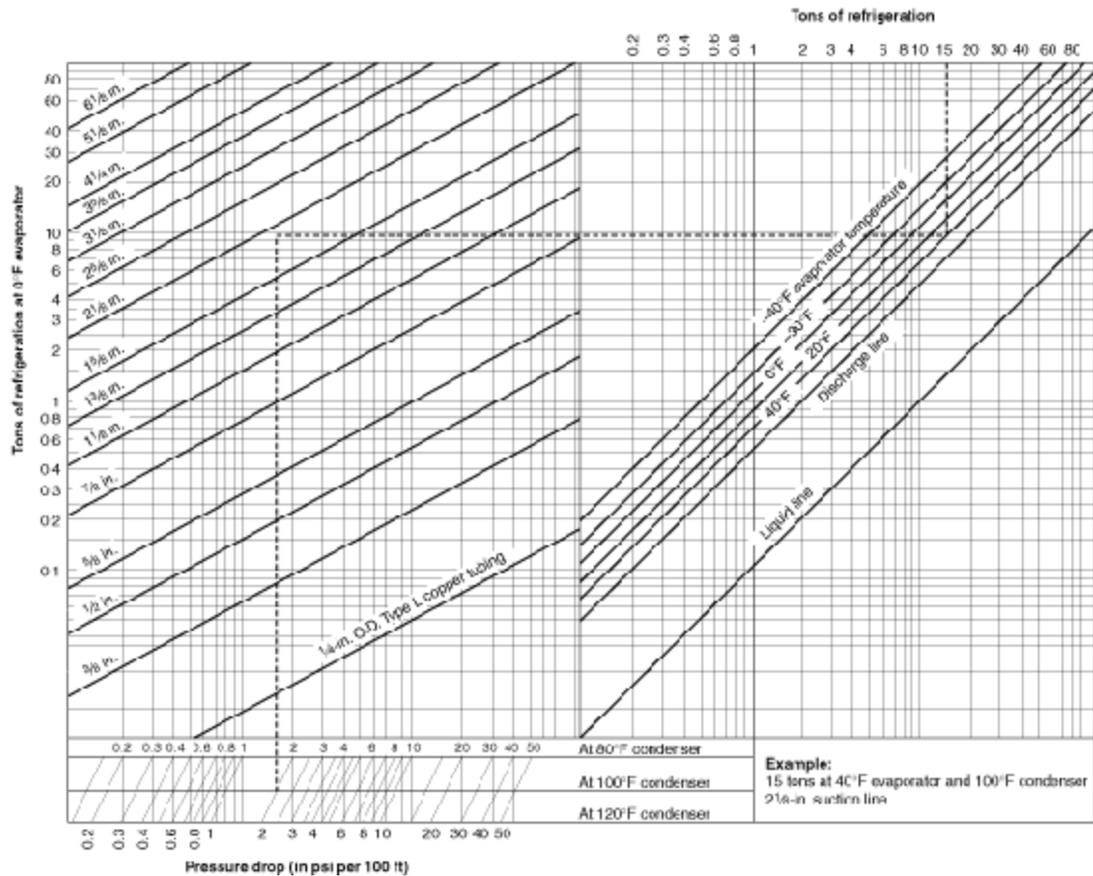
Figure 66F17 Pressure Drops in Refrigerant Lines Freon 12. Figured for type L copper tubing. For iron pipe subtract 1/8" from copper tubing size to find nominal iron pipe size. Multiply copper pressure by 16.
