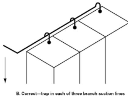
Figure 66F08B Same refrigerators as in Figure 66F08A, but with trap in each of the three branch suction lines (Right).
