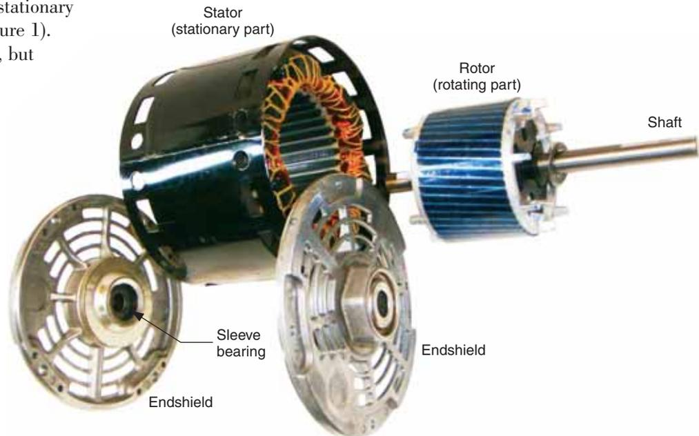
Figure 1. Typical ac induction electric motor
