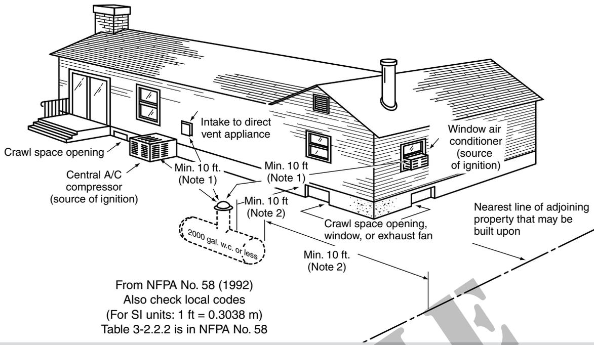
Note 1: The relief valve, filling connection, and liquid level gauge vent connection at the container must be at least 10 ft from any exterior source of ignition, openings into direct-vent appliances, or mechanical ventilation intakes. Refer to Note (d) under Table 3-2.2.2.
