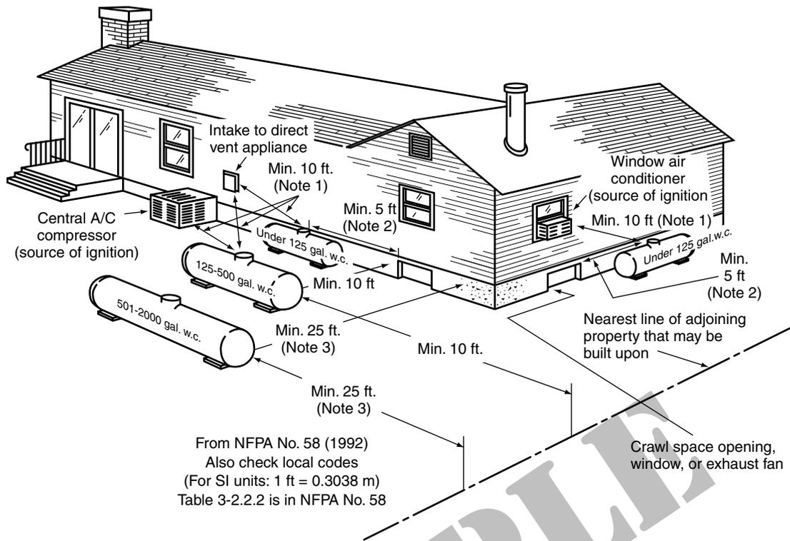
Note 1: Regardless of its size, any ASME tank filled on site must be located so that the filling connection and fixed liquid level gauge are at least 10 ft from any external source of ignition (i.e., open flame, window A/C, compressor, etc.), intake to direct vented gas appliance or intake to a mechanical ventilation system. Refer to Note (b) (3) under Table 3-2.2.2.
