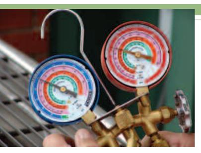
and/or oil in the system should be dedicated to R-410A systems. In addition, a dedicated manifold gauge set should be used with R-410A equipment. Manifold gauge sets exist that can handle both R-410A and R-22. However, if using a dual-refrigerant manifold gauge set, it is recommended that it is only used with one refrigerant.
