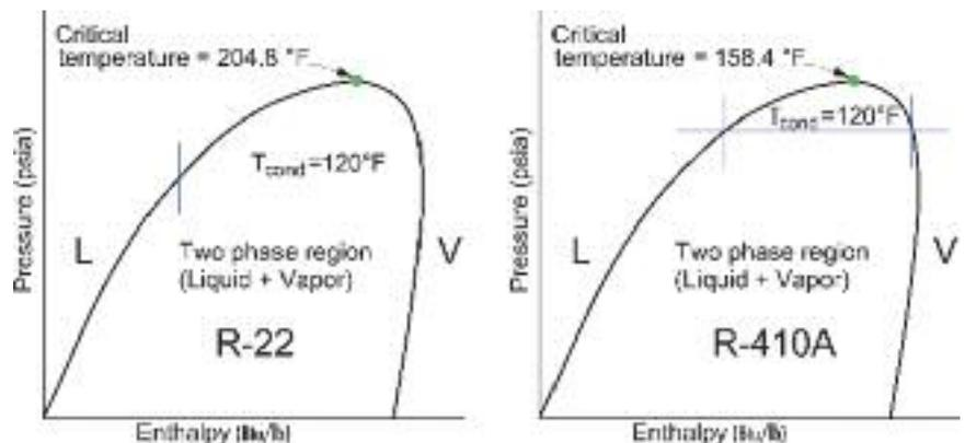
**Figure 1** This illustration highlights pressure-enthalpy schematics, showing how at higher ambient temperatures, R-410A has less room to work with in the two-phase region than does R-22. This is a key consideration in replacement, especially in areas where the system's design ambient condition is often high.
