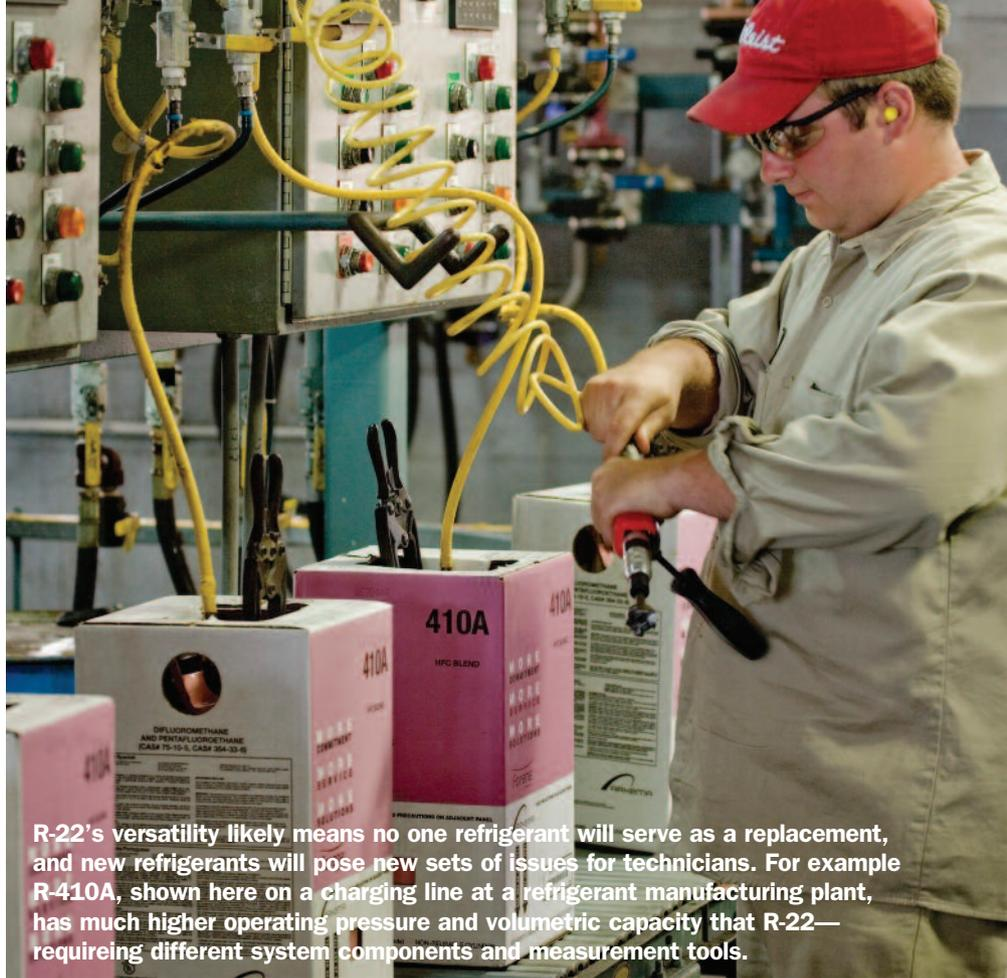
R-22's versatility likely means no one refrigerant will serve as a replacement, and new refrigerants will pose new sets of issues for technicians. For example R-410A, shown here on a charging line at a refrigerant manufacturing plant, has much higher operating pressure and volumetric capacity than R-22—requiring different system components and measurement tools.
