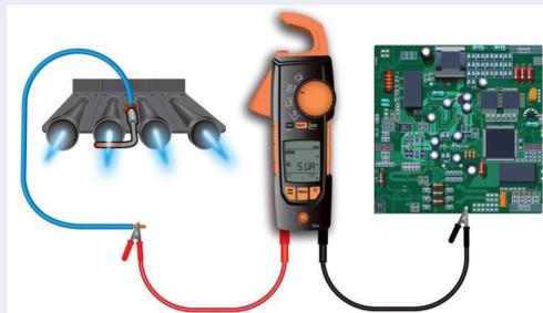
Because the flame rectification (sensing) circuit requires current flow through the burner ground, that is a practical place to start.
