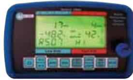
automatically calculate superheat and subcooling; and dual temperature probes to easily read SH, SC and  $\Delta T$ . For mechanics in high-altitude areas, the DRSA 1250 can be zeroed manually. Circle 7 on the reader service card.
