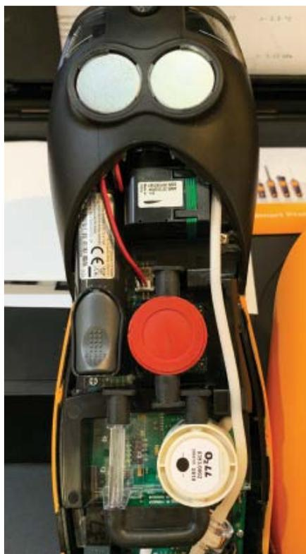
⚡ This analyzer has room for a third (NO) sensor to be installed.
