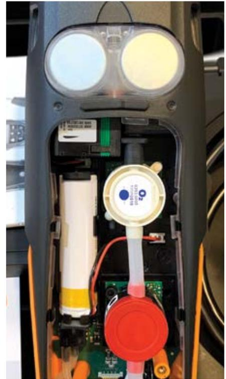
⚡ Note the magnetic disks above the battery-sensor bay. They allow the analyzer to mount to the appliance, yielding hands-free operation.
