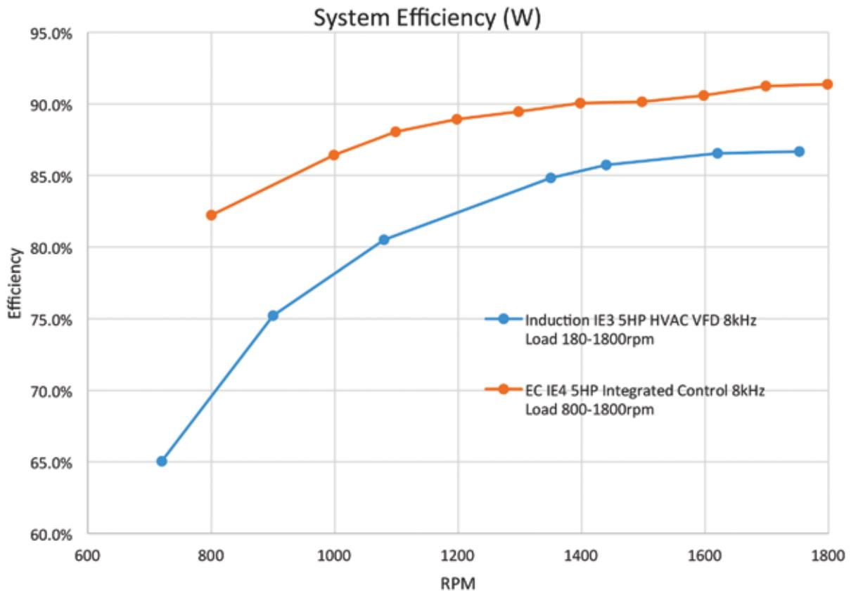
^ Figure 1 Advanced EC motor designs with IE4 efficiency ratings and tuned VFD experience less efficiency loss at low speeds than traditional induction motors.
