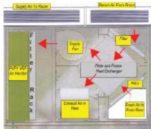
« Diagram of a plate and frame heat exchanger-enthalpy core.
