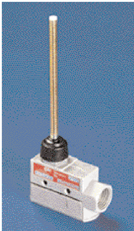
Figure 4 Here's a typical interlock safety switch, which is placed on the hvac system duct access panels and on doors to prevent accidental UV exposure.
