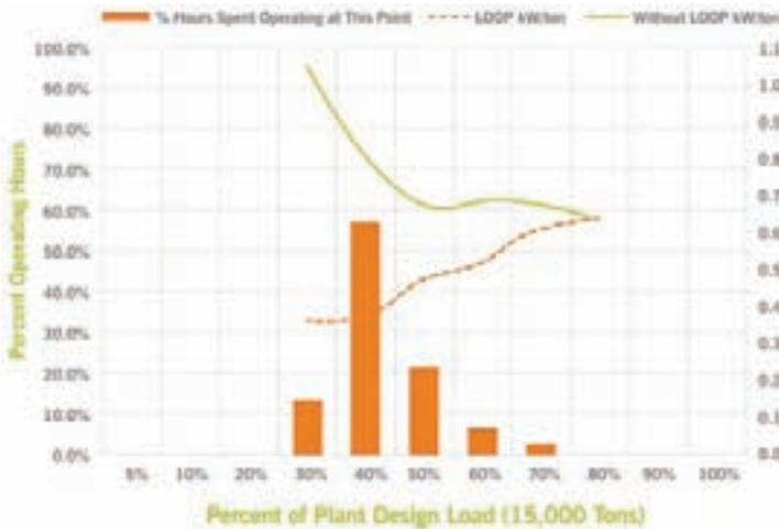
Figure 9: Monthly plant efficiency reports include graphical representation of key operating statistics. This Performance Summary shows that for about 70% of the total run hours, this plant was running between 30% to 40% of design load where the performance ranged from 0.32 to 0.35 kW/ton.
