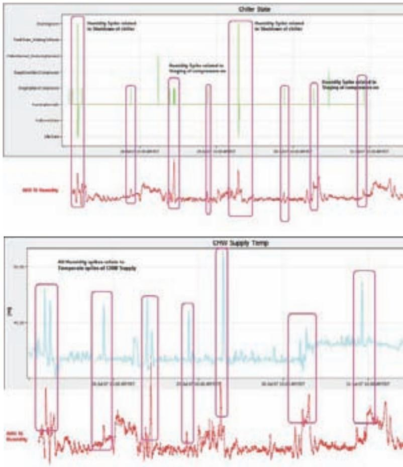
*OptimumMVM Case Study: In this example, custom charts were created to correlate the on/off staging of the chiller and the chilled water supply temperature with humidity levels. Using these charts, the chain of events that caused the periodic rise in humidity levels was easily diagnosed.*
