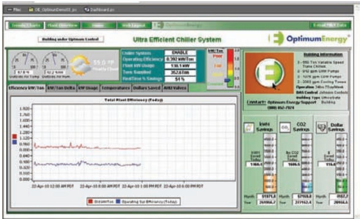
Figure 6: The OptimumMVM Dashboard view provides an at-a-glance overview of plant performance, including real time operating efficiency, daily and monthly dollars saved, and CO<sub>2</sub> reduction.
