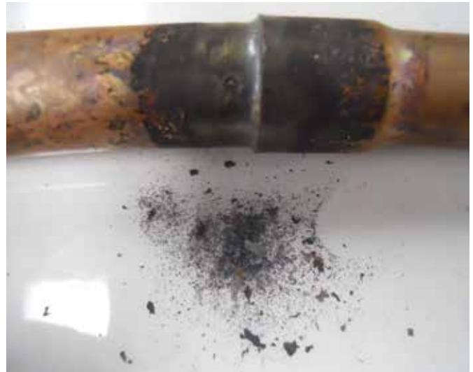
⤴ Inside oxidation scale from 5/8-in. tube.
