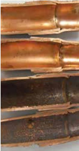
⤴ Nitrogen-purged tubes at the top compared to the bottom tubes that did not receive nitrogen purging.
