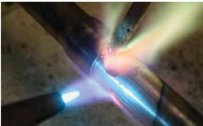
⤴ **Image 3.** When heated, the coating on flux-coated rods will liquefy and move into the joint before the braze alloy melts and follows. This makes for a tight connection with minimal flux inside the joint.
