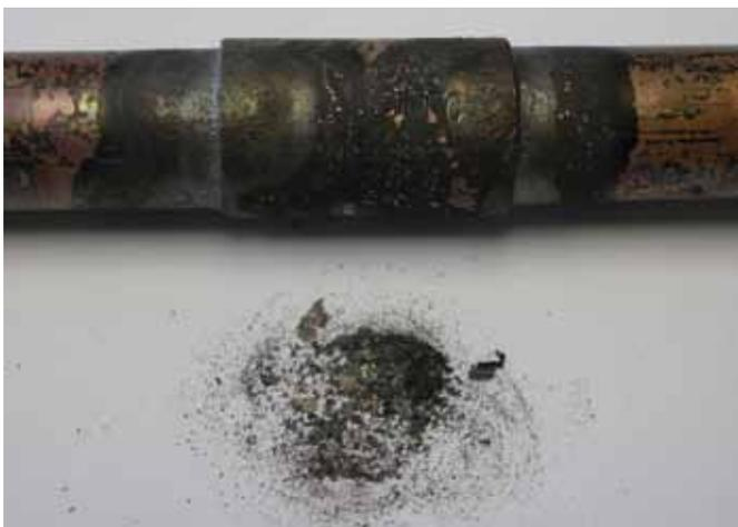
⤴ **Image 4.** Brazing can cause copper to oxidize, forming flakes of “scale” metal like the ones shown from this 5/8-in. outside-diameter fitting braze job. A nitrogen purge can help prevent this problem.
