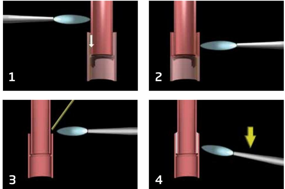
**Step 3. Heat**—The most frequent cause of poorly brazed joints is incorrect heating. The goal is simple: heat both tube and fitting to evenly bring them to brazing temperature, and do so before you apply the braze rod. Here is a suggested approach to accomplish that goal (see the illustrations in Figure 1):
