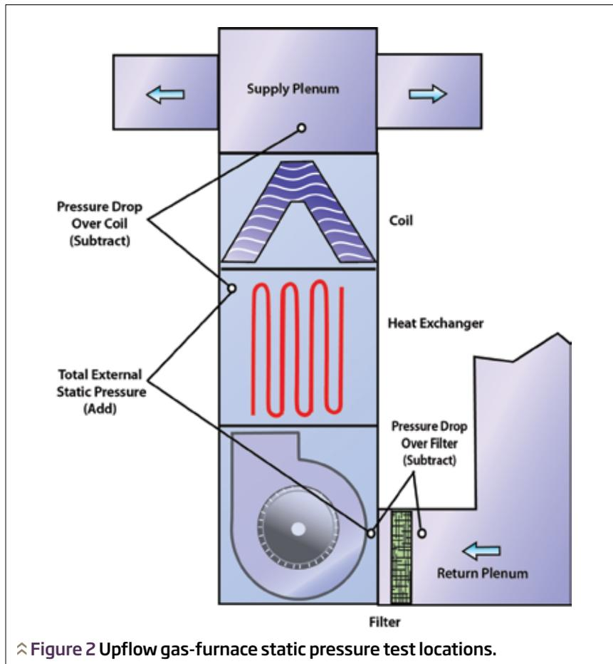
Figure 2 Upflow gas-furnace static pressure test locations.
