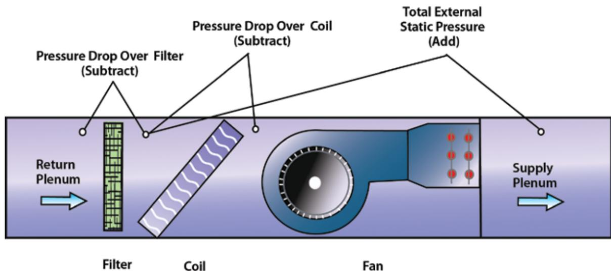
⚡ Figure 1 Horizontal air-handler static pressure test locations.
