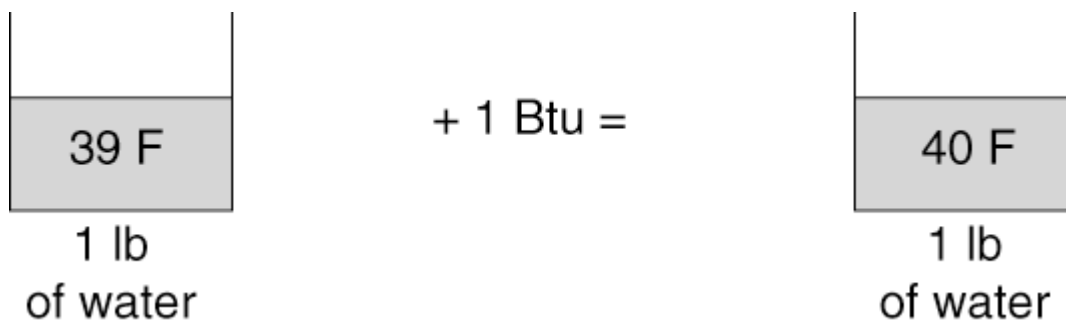
FIGURE 2F53 The British thermal unit or Btu is defined as the amount of heat needed to raise the temperature of one pound of water one degree F.
