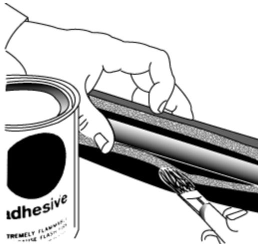
Figure 13 Push the insulation down.
